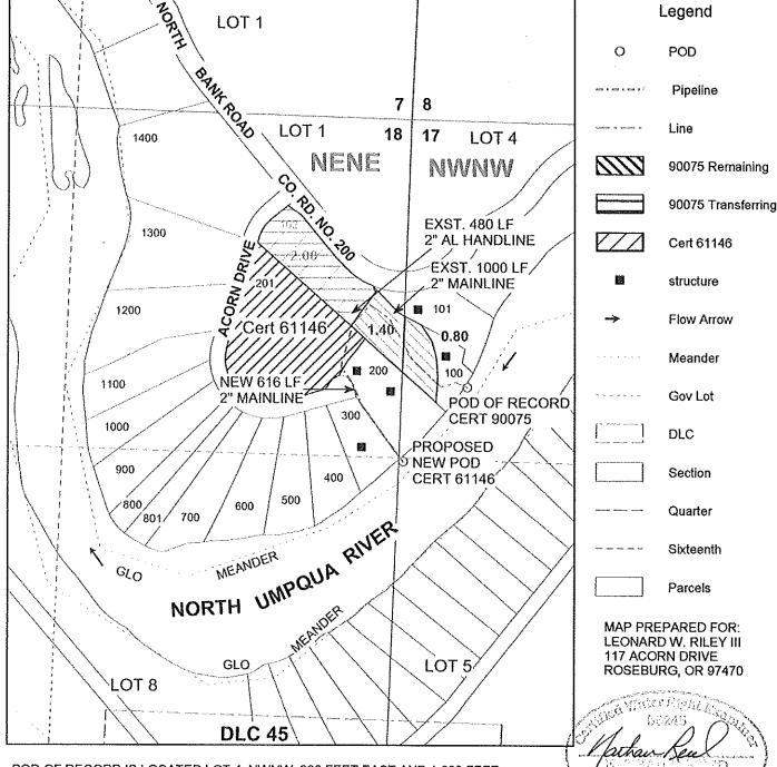
POD OF RECORD IS LOCATED LOT 4, NWNW, 380 FEET EAST AND 1,000 FEET SOUTH OF THE NW CORNER OF SECTION 17.
