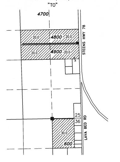
WELL 2 (HARN 51923) LOCATED IN THE SE 1/4 SE 1/4 SECTION 25, T26S R33E, W.M. AND 30 FEET NORTH AND 1320 FEET WEST FROM THE SE CORNER OF SECTION 25.
