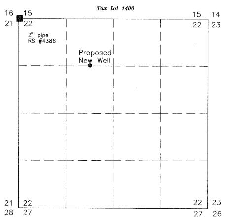
Proposed new well is located in the NE1/4NW1/4 of Section 22 and located 1997' East and 1327' South of the NW corner of Section 22, T39S R19E
