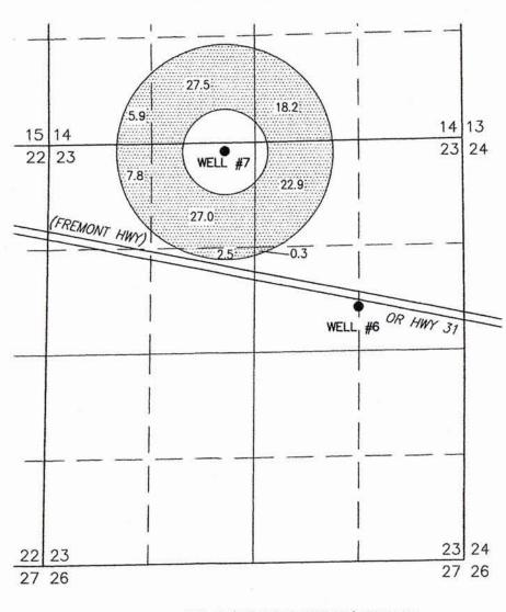
WELL #7 (LAKE 52463 PROPOSED) IN THE NE 1/4 NW 1/4 SECTION 23, T34S R19E, W.M. LOCATED 105 FEET SOUTH AND 3000 FEET WEST FROM THE NE CORNER OF SECTION 23.
