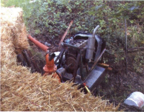
Diesel pump used at POD for sprinklers - Straw bales to minimize noise May 22, 2013 at 5:17:40 PM
