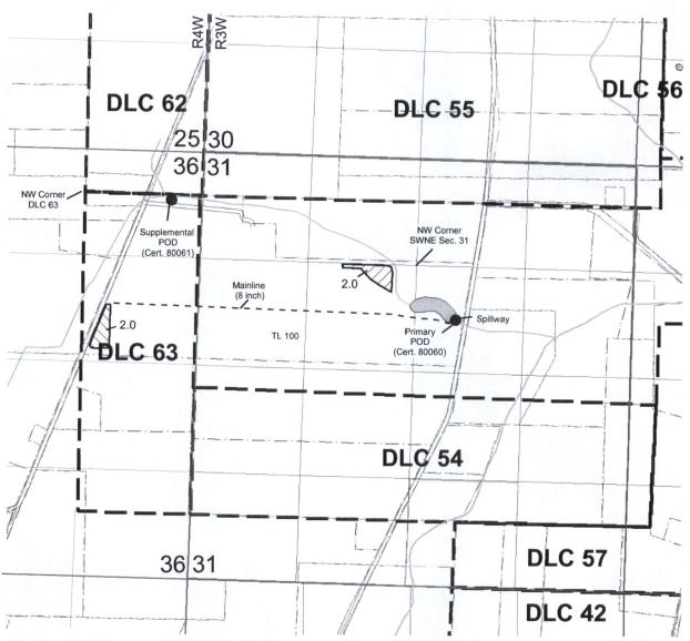
Primary Cert. 80060 POD is located 660'S and 500' E from the NW corner of SWNE Section 31 Supplemental Cert. 80061 POD is located 100'S and 990' E from the NW corner of DLC 63
