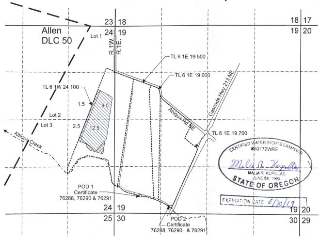
Authorized POD 1 is located 4,790 feet south and 720 feet east from the NW corner, Section 19. Authorized POD 2 is located 5,090 feet south and 1,580 feet east from the NW corner, Section 19.
