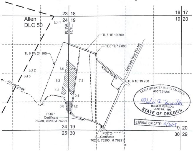
Authorized POD 1 is located 4,790 feet south and 720 feet east from the NW corner, Section 19. Authorized POD 2 is located 5,090 feet south and 1,580 feet east from the NW corner, Section 19.
