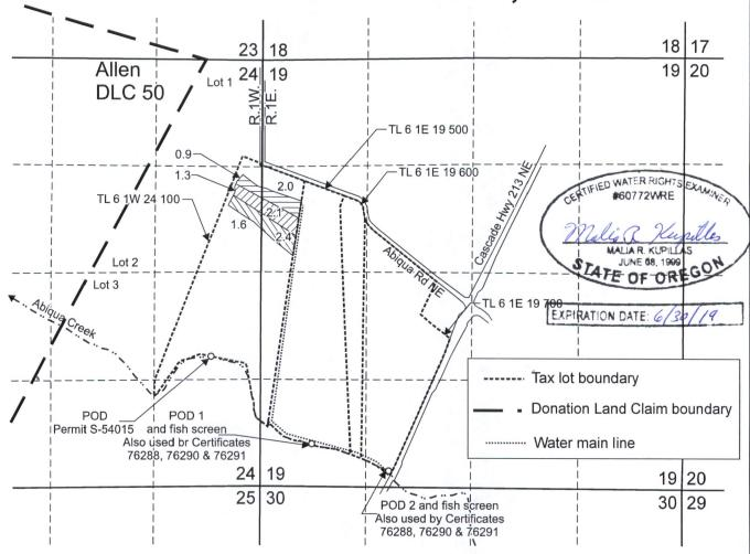
POD (Permit S-54015) is located 3,680 feet south and 640 feet west from the NE corner, Section 24.
