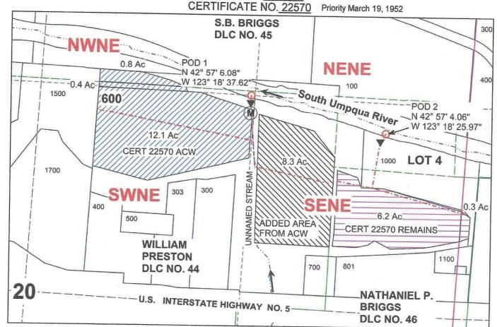
POD 1 IS LOCATED 1333 FEET NORTH AND 1343 FEET EAST FROM THE C1/4 CORNER OF SECTION 20 AS PROJECTED WITHIN DLC NO. 44. POD 2 IS LOCATED 1159 FEET NORTH AND 528 FEET WEST FROM THE E1/4 CORNER OF SECTION 20 AS PROJECTED WITHIN G.LOT 4.
