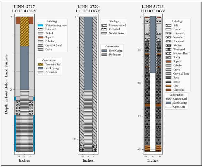
The depth and construction of the three authorized POA wells (two shown above) versus that of the proposed POA well (at right) are vastly different and designed to produce from different aquifer systems.
