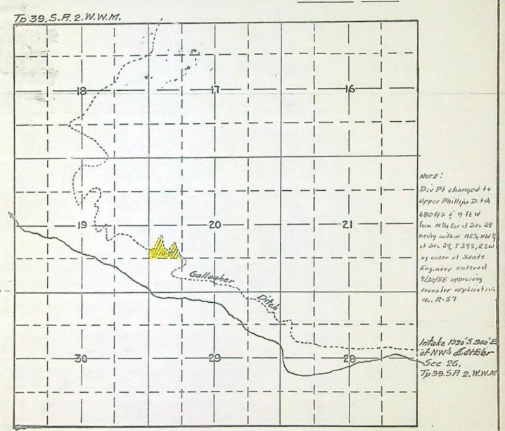
Map made from notes in the field from an actual survey by C. Frank Phodes, the same correctly showing the lands to be irrigated, together with streams and ditches in the immediate vicinity. compiled by
