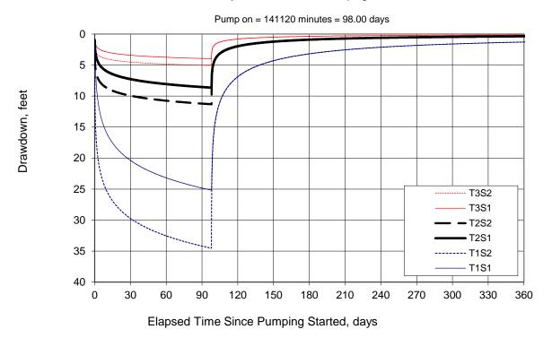
Radial distance, r = 600 ft [approximate distance from To-POA to CLAC 18564] Pumping time,  $t_{pump} = 98$  days [approx. time to exhaust duty under Permit G-18861 at 0.4 cfs] Pumping rate, Q = 0.473 cfs [maximum combined rate under T-14377 and T-14560] Transmissivity, T1 = 800 ft<sup>2</sup>/d | T2 = 2,800 ft<sup>2</sup>/d | T3 = 6,800 ft<sup>2</sup>/d [Pumping Test Reports] Storativity, S1 = 0.001 | S2 = 0.0001 [Conlon et al., 2005]
