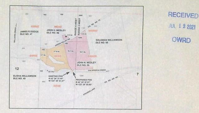
EXISTING POD IS LOCATED 2630 FEET NORTH AND 2400 FEET EAST FROM THE S1/4 CORNER OF SECTION 12 AS PROJECTED WITHIN DLC NO. 46. PROPOSED POD TO BE LOCATED 2630 FEET NORTH AND 2500 FEET EAST FROM THE S1/4 CORNER OF SECTION 12 AS PROJECTED WITHIN DLC NO. 46.
