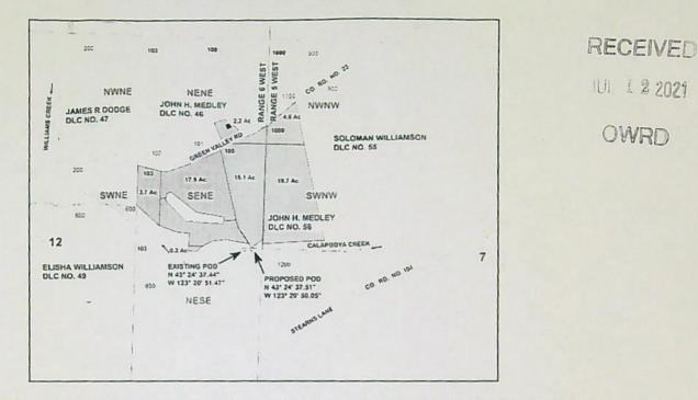
EXISTING POD IS LOCATED 2630 FEET NORTH AND 2400 FEET EAST FROM THE S1/4 CORNER OF SECTION 12 AS PROJECTED WITHIN DLC NO. 46. PROPOSED POD TO BE LOCATED 2630 FEET NORTH AND 2500 FEET EAST FROM THE S1/4 CORNER OF SECTION 12
