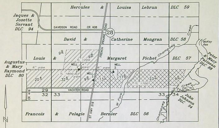
Existing Well #1 (to be replaced): 1340' N & 2300' E of SW Cor Pichet DLC No. 57 Proposed Well #3 (replacement well): 905' N & 2995' E of SW Cor Pichet DLC No. 57 Existing Well #2 (to remain): 1270' N & 3900' E of SW Cor Pichet DLC No. 57
