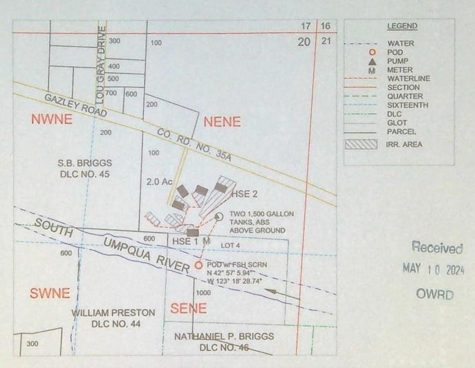
POD IS LOCATED 1408 FEET SOUTH & 723 FEET EAST OF NE CORNER OF SECTION 20 AS PROJECTED WITHIN GLOT 4.
