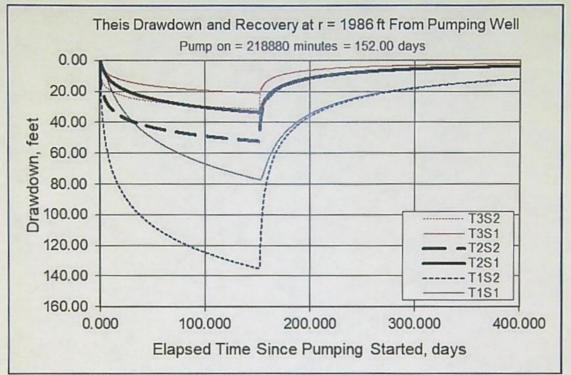
Radius, r=1,986 ft [approximate distance from "Well 2" (MARI 51725) to MARI 1061] Pumping time, t=152 days [approximate time to exhaust combined duty at max combined rate] Pumping rate, Q=2.59 cfs [total combined rate under all applicable rights] Transmissivity: T1=700 ft<sup>2</sup>/day; T2=2,200 ft<sup>2</sup>/day; T3=4,000 ft<sup>2</sup>/day [Pumping Test Reports] Storativity: S1=0.003; S2=0.0003 [Conlon et al 2005]
