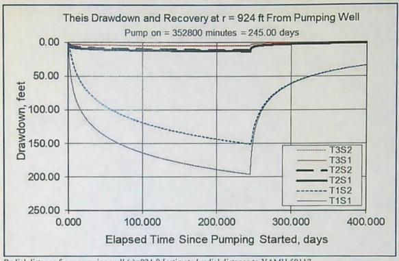
Radial distance from pumping well (r)=924 ft [estimated radial distance to YAMH 59117 Pumping Rate (Q)= 0.18 cfs (81 gpm)\*
