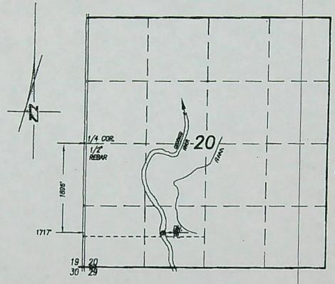
NOTE: THE ABANDONED DIVERSION POINT LOCATED 744.2' SOUTH BY 321' EAST OF W.1/4 CONNER OF SECTION 8, T.15S., R.16E.,W.M. (PEOPLE'S IRRIGATION CO.)
