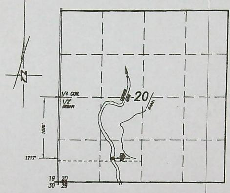
NOTE: THE ABANDONED DIVERSION POINT LOCATED 744.2' SOUTH BY 321' EAST OF W.1/4 COMMER OF SECTION 8, T.15S., R.16E.,W.M. (PEOPLE'S IRRIGATION CO.)
