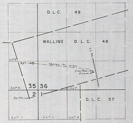
Spring located 1600'N. \$ 170' E. from S. W. Cor. Walling D.L.C. 48
