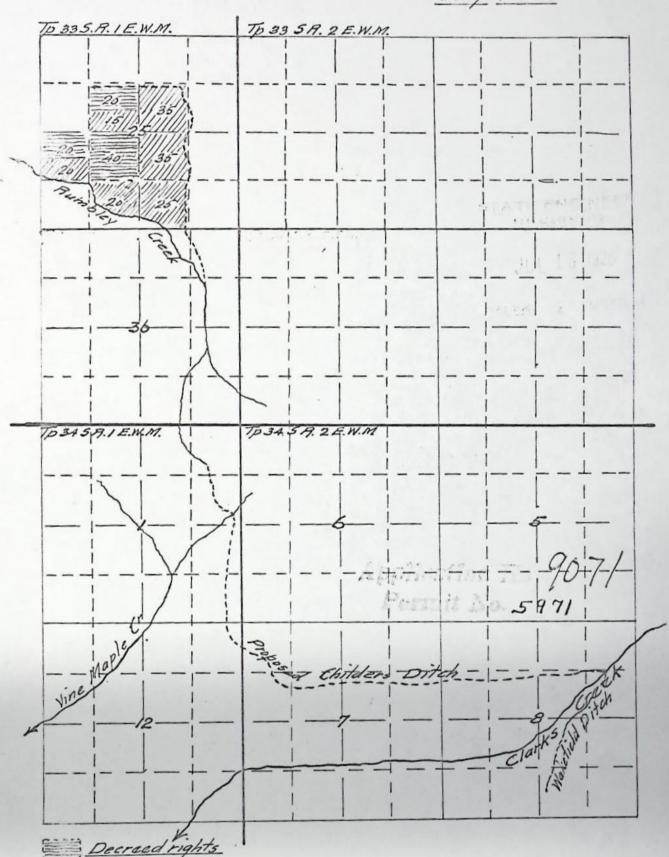
Will Irrigation New by Mr Childers, showing approximate location of ditch and correctly showing lands to be irrigated to-gether with streams and ditches in immediate vicinity. Fred. N. Cummings. C.E. compiled by.
