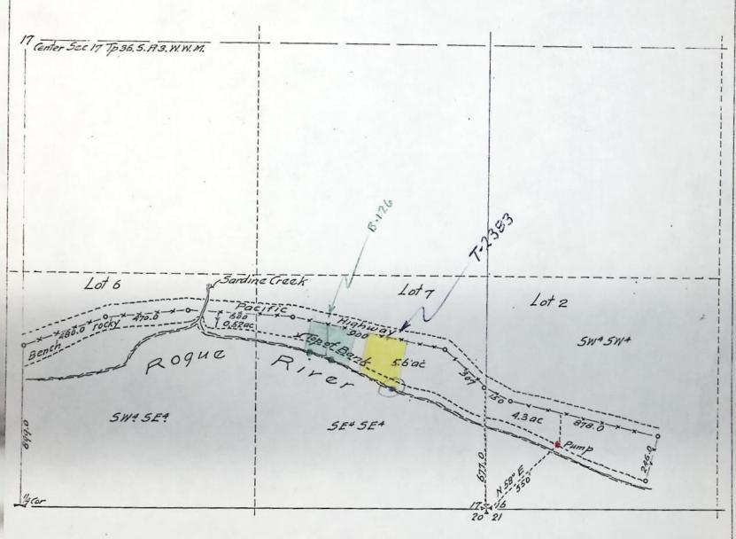
Map made from notes taken in the field in Survey made by C.I. Boyden County surveyor. The same showing correctly Lands to be irrigated, together with streams and ditches in immediate vicinity Compiled by.
