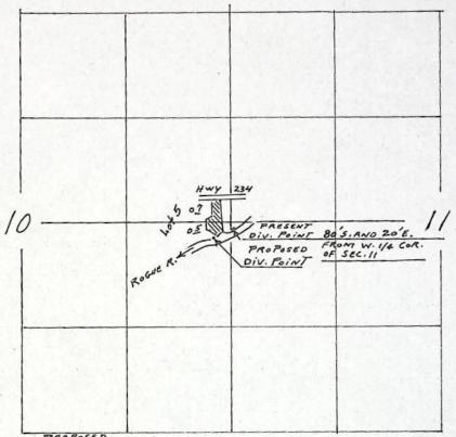
PROPOSED DIVERSION POINT IS LOCATED 200'S. AND 200'W. FROM THE E. 1/4 COR. OF SEC. 10
