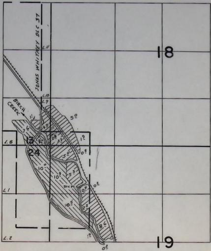
DIVERSION POINT I LOCATED 1140'S. \$ 790'E. FROM NW COR SEC 19 DIVERSION POINT Z LOCATED 320'N. \$270 W. FROM NW COR SEC 19
