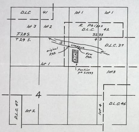
New P.O.D. located 480 ft. S. and 985 ft. W. from the N.E. Corner of Section 4.
