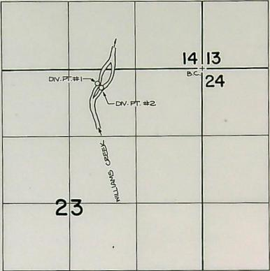
DIV. PT. #1 19 LOCATED 300'S. AND 2080'W., DIV. PT. #2 IS LOCATED 350'S. AND 2010'W., BOTH FROM THE N.E. CORNER OF SECTION 23.
