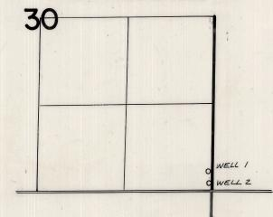
WELL I LOCATED 290' N. \$ 50'W. FROM SE COR SEC 30, T. 4N. R. 21E. W.M. WELL Z LOCATED 100' N. \$ 40' W. FROM SE COR SEC 30, T. 4N. R. 21E. W.M. WELL 3 LOCATED 1970'S. \$ 790' W. FROM NE COR SEC 4, T. 3N. R. 21E. W.M.
