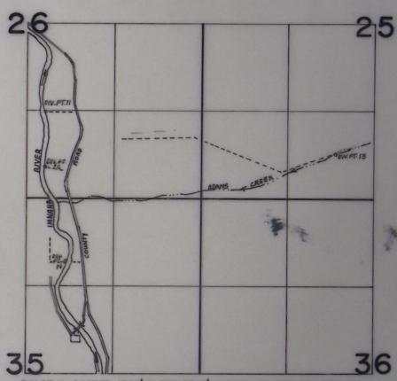
DIV.PT.II LOCATED 1300' N. AND 2360' W. FROM SE. SEC. COR. SEC. 26 DIV.PT.I2 LOCATED 460' N. AND 2370'W. FROM SE. SEC. COR. SEC. 26 DIV.PT.I3 LOCATED 770' N.AND 2050' E. FROM S.W. SEC. COR. SEC. 25 DIV.PT.I4 LOCATED 940' S. AND 2050' W. FROM NE. SEC. COR. SEC. 35
