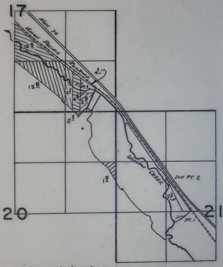
DIV. Pr. 1 240'S & 1120'W FROM CENTER Sec. 21 DIV. Pr. 2 1950'S & 1490'E. FROM NW COR. SEC. 21 DIV. Pr. 3 600'N. & 680'W. FROM SE COR. SEC. 17
