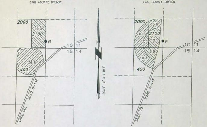
WELL #1 (LAKE 1385) AUTHORIZED & LOCATED IN THE SW 1/4 SE 1/4 SECTION 10, T28S R16E, W.M. LOCATED 310 FEET NORTH AND 1340 FEET WEST FROM THE SE CORNER OF SECTION 10.
