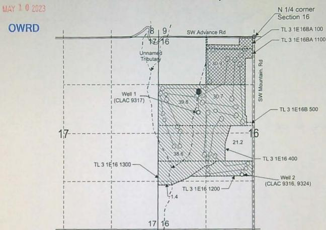
Well 1 (CLAC 9317) is located 2,050 feet south and 1,560 feet west from the N 1/4 corner, Section 16.
