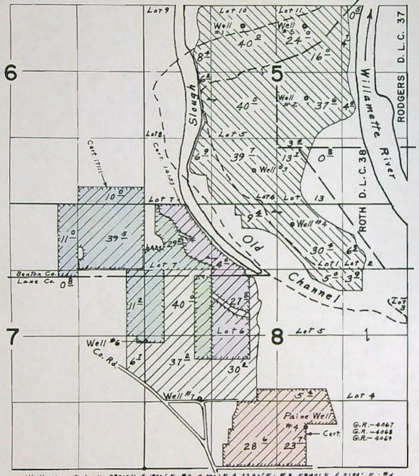
Wells located: #1,8830'N. \$ 1970'E; #2,7,380'N. \$ 3240'E; #3,5940'N. \$ 2180' E.; #4, 4860' N. & 2950' E.; #5, 8,830' N. & 3,220' E.; #6, 2540' N. & 30' E.; #7, 1380' N. & 1100' E., Payee Well # 4, 800' N. & SESO' E.; all from Common Corner to Sections 7,8, 17 \$ 18
