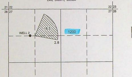
21.3 ACRES PRIMARY GROUND WATER RIGHTS FROM CERTIFICATE #90483 (G-7174) POA 5 TRANSFERRED AS SHOWN. WELL 2 (LAKE 186) WELL IN NW 1/4 NW 1/4 OF SECTION 27, T25S R15E, W.M. LOCATED 1309 FEET SOUTH AND 1562 FEET WEST FROM N 1/4 CORNER.
