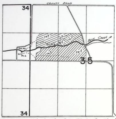
DIV. P. I LOC: 460 N. + 250 W. FROM E'4 COR. SEC 34 - TONEY-BLIE DITCH DIV. P. Z LOC: 400'N. & 400' W. FROM EV4 COR. SEC 34 - FAVORITE DITCH DIV. Pr. 3 Loc: 710'N. + 1130'E. FROM WILL COR. SEC 35 - TONEY DITCH
