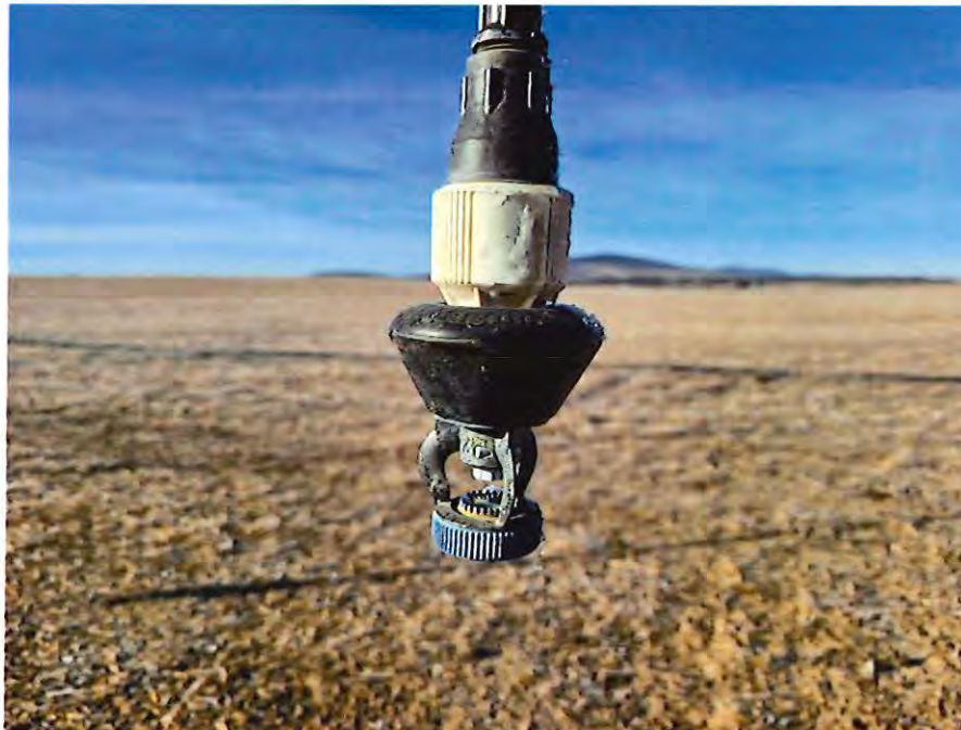
Typical Pivot Nozzle, Section 18
