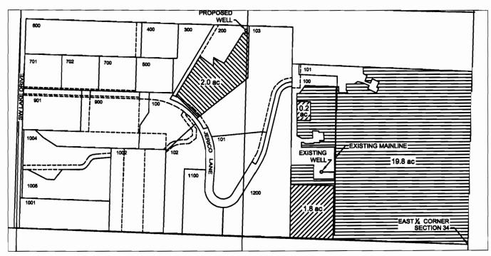
EXISTING WELL: LOCATED 2300' SOUTH AND 870' WEST FROM NE CORNER OF SECTION 34 PROPOSED WELL: LOCATED 1490' SOUTH AND 1330' WEST FROM NE CORNER OF SECTION 34
