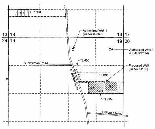
Authorized Well 1 (CLAC 02569) is located 570 feet south and 2,420 feet west from the NE corner of Section 19. Authorized Well 2 (CLAC 02574) is located 530 feet south and 670 feet west from the NE corner of Section 19. Proposed Well (CLAC 61132) is located 2,090 feet south and 860 feet west from the NE corner of Section 19.
