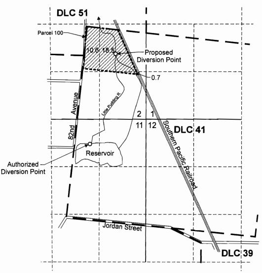
Authorized diversion point is located 690 feet S. and 1,070 feet E. from the N 1/4 corner, Section 11. Proposed diversion point is located 760 feet S. and 790 feet E. from the NW corner, DLC 41.
