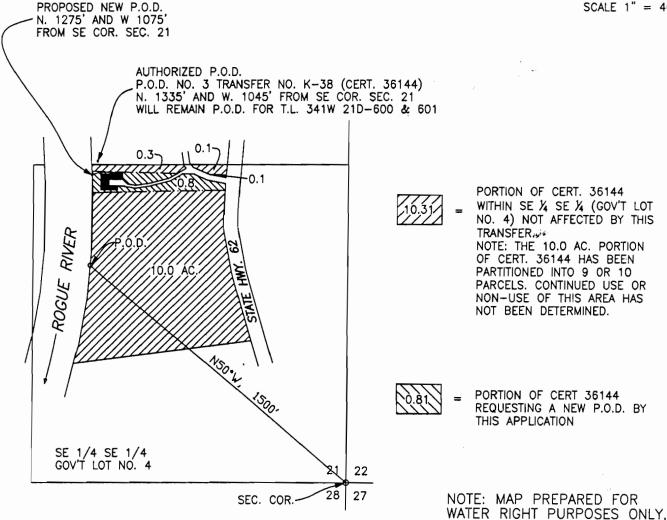
MAP TO ACCOMPANY AN APPLICATION FOR A TRANSFER OF WATER RIGHT, CHANGE IN POINT OF DIVERSION
