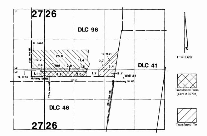
Well is located 578'N & 924'E from the SW corner of DLC 96. Well #1 is located 100'N & 350'E from the NE corner of DLC 46.
