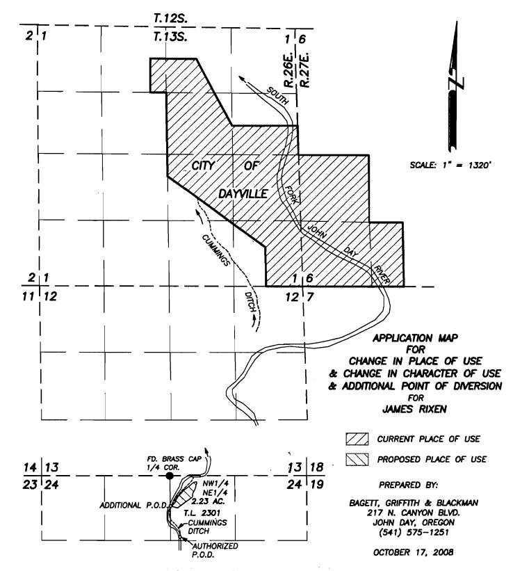
ADDITIONAL POD IS 600' SOUTH & 25' WEST OF THE N1/4 CORNER SECTION 24, T.13S., R.26E., W.M. AUTHORIZED POD IS 1200' SOUTH & 140' EAST OF THE N1/4 CORNER SECTION 24, T.13S., R.26E., W.M.
