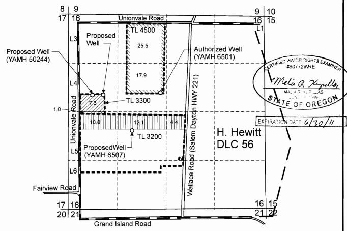
Authorized Well (YAMH 6501) is located 1890 feet south and 2230 feet east from the NW corner of DLC 56. Proposed Well (YAMH 6507, Shelburne Transfer) is located 2910 feet south and 1460 feet east from the NW corner of DLC 56.
