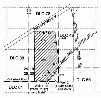
Well 1 (YAMH 2912) is located 820 feet south and 700 feet west from the SW corner, A & P Smith DLC 48. Well 2 (YAMH 54354) is located 200 feet south and 660 feet west from the SW corner, A & P Smith DLC 48.
