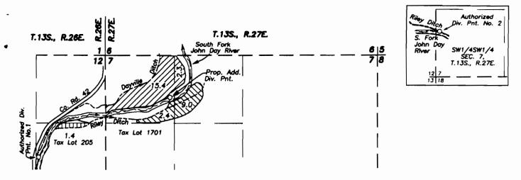
Proposed Additional Diversion Point is 830' S. and 1260' E. of the NW Cor. Sec. 7, T.13S., R.27E. Authorized Diversion Point No.1 (Dayville Ditch) is 1980' S. & 1310' W. from the NE Cor. Sec. 12, T.13S., R.26E. Authorized Diversion Point No.2 (Riley Ditch) is 900' N. & 70' E. from the SW Cor. Sec 7, .T.13S., R.27E.
