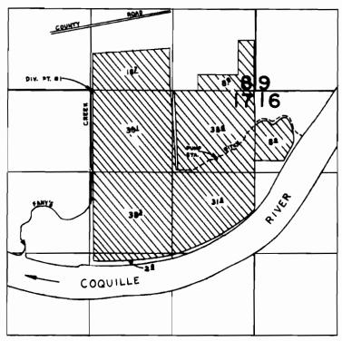
DIV. PT 0: LOCATED 16'E. FROM N. 1/4 CORNER SECTION 17 DIV. PT 0: LOCATED 15'N. \$ 25' E. FROM N. 1/18 CORNER SECTION 17 PUMP STA. LOCATED 1,090'S. \$ 630' W. FROM N.E. CORNER SECTION 17
