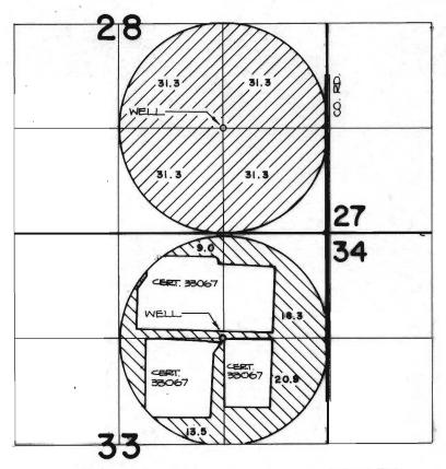
G-9373 THE WELL IS LOCATED 1320 FT. N. AND 1300 FT. E. FROM THE 5.1/4 CORNER OF SECTION 28.
