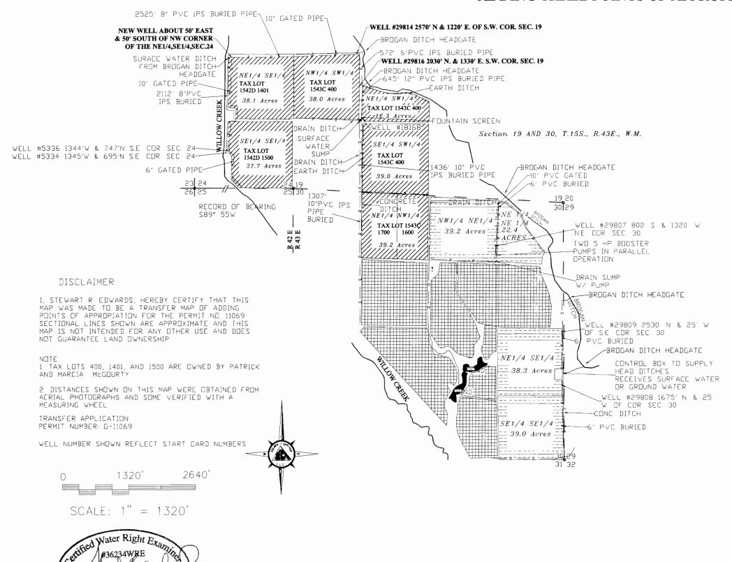
LEGEND GOVERNMENT CORNER LAND INCLUDED IN PERMIT G-11069 ADDITIONAL LAND INCLUDED IN PERMIT G-12581 LAND INCLUDED IN OTHER WATER RIGHTS CONC LINED DITCH EARTHEN DITCH DRAIN DITCH BURIED — в — в — в — в — PIPE LINE GATED PIPE DRAIN PIPE -&- WELL WELL PUMP DRAIN SUMP
