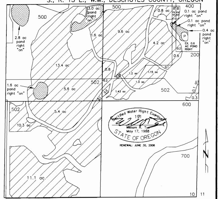
I, WILLIAM R. TYE, CERTIFIED WATER RIGHT EXAMINER IN THE STATE OF OREGON, HEREBY CERTIFY THE ABOVE APPLICATION MAP WAS PREPARED UNDER MY DIRECT SUPERVISION. THE PREPARATION OF THIS MAP IS FOR THE PURPOSE OF IDENTIFYING THE LOCATION OF THE WATER RIGHT ONLY AND HAS NO INTENT TO PROVIDE DIMENSIONS OR LOCATIONS OF PROPERTY OWNERSHIP LINES.
