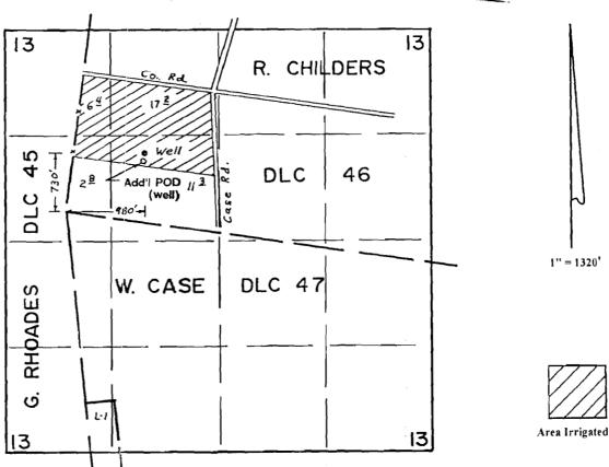
Auth. POD is located 730'N & 980'E from the SW corner of DLC 46. Add'l POD is located 680'N & 980'E from the SW corner of DLC 46.
