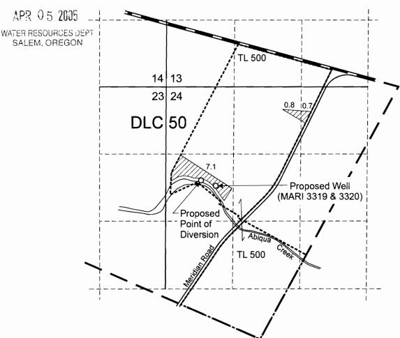
Proposed Well (MARI 3319 & 3320) is located 690 feet north and 990 feet east from the W 1/4 Corner, Section 24.
