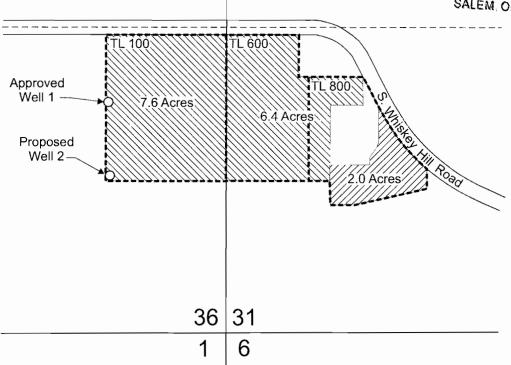
Approved Well 1 is located 1,000 feet north and 510 feet west from the SE corner of Section 36. Proposed Well 2 is located 700 feet north and 510 feet west from the SE corner of Section 36.
