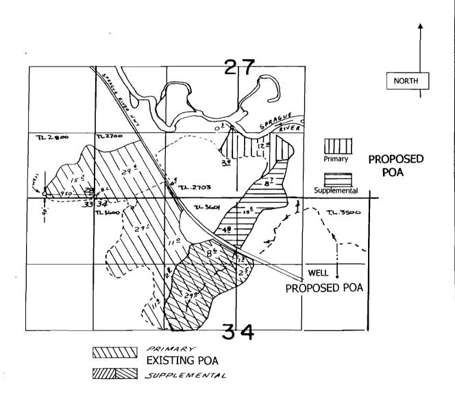
PROPOSED POINT OF APPROPRIATION: 1550'S & 4870'E from SW cor section 27
